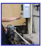
Hydrant being assembled using a custom made power torque wrench complete with electric eye. This is what ensures proper torque with precise alignment of drain port on every hydrant.
